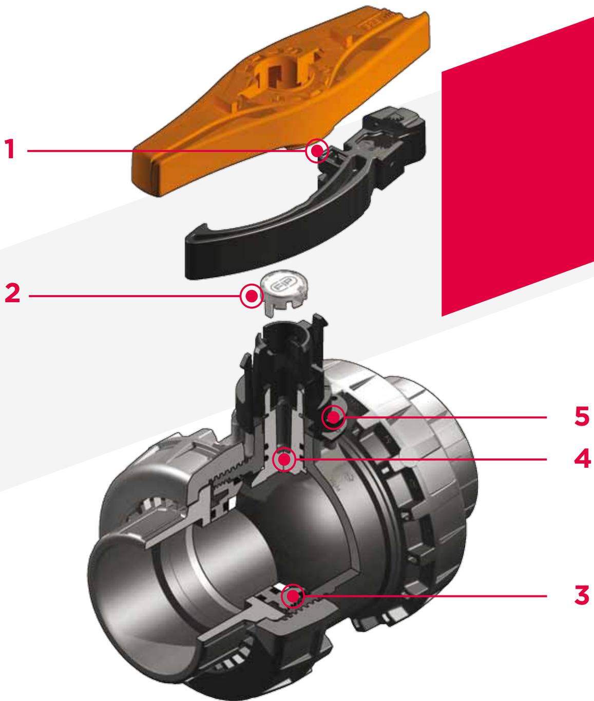
**1 Innovative Easyfit quick release handle** made up of a central hub firmly coupled with the stem valve and **dual spoke grip** that can be released from the hub with a simple operation and used as a **ball seat adjustment tool** and as a **union nut tightening tool** thanks to the hooked insert that, perfectly adapting to their external profile, allows the handle to transform into a wrench to control union nut rotation
