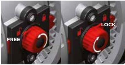
Rotate the button to the left, pointing the arrow on the open lock to unlock DUAL BLOCK®: the valve union nuts are free to rotate clockwise and counter-clockwise. Rotate the button to the right, pointing the arrow on the closed lock to lock DUAL BLOCK®: the valve union nuts are blocked in the desired position.
