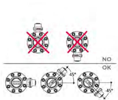
Make sure that the valves installed on the system are suitably supported for their weight.
