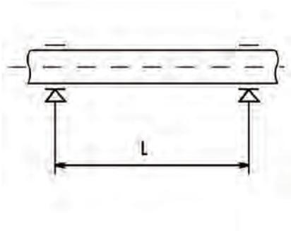
The installation of thermoplastic pipe systems requires the use of support clips to prevent flexing and the resulting mechanical stresses. The distance between the clips depends on the pipe material, SDR, surface temperature and the density of the conveyed fluid. Before installing the clips, check the distances reported in the table below, as provided for by guidelines DVS 2210-01 for water pipes.
