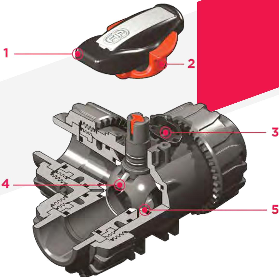
**1** Ergonomic HIPVC handle equipped with removable tool to adjust the ball seat carrier. Possibility of installing the **LTKD stroke limiter** (available as an accessory) that permits ball and handle rotation only for set opening and closing angles at 90° or 180°
